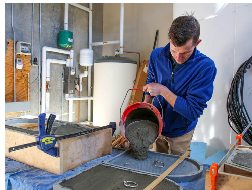
Above: Kodi Bowers '20 pours mixed concrete into forms to create hellbender nesting boxes
